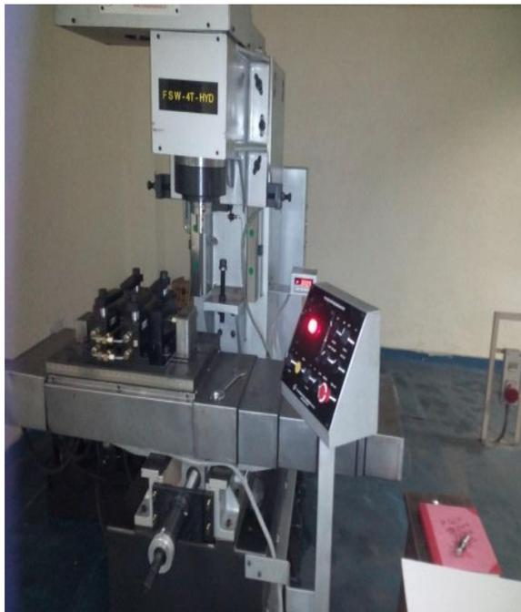
Figure 3.1: Friction stir welding / processing machine ( DTU)
